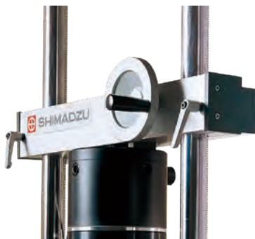
The crosshead can be positioned easily using a manual handle and lever.
