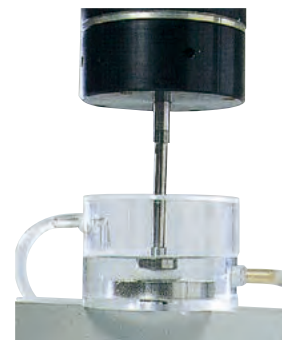
The thermostatic water immersion test unit is ideal for testing biological material and implants.
