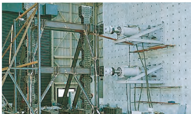
Loading Test for Steel Structural Members \pm 1000 kN
