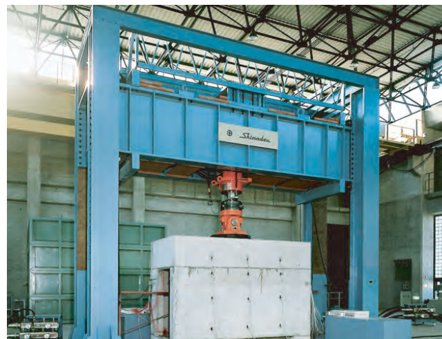
Compressive Fatigue Test of Steel Reinforced Concrete Manhole Covers \pm 1000 kN
